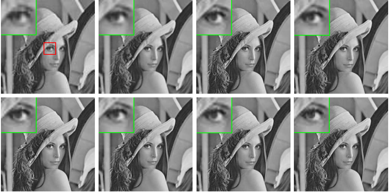
Fig. 3. Results for the Lena input image of size 128 \times 128 magnified by a factor of m = 2 . Top row: low-resolution input, bicubic interpolation, Yang et al. 's method [16], and Zeyde et al. 's method [17]. Bottom row: Chen et al. 's method [21], Dong et al. 's method [27], our method, and the original HR image.
